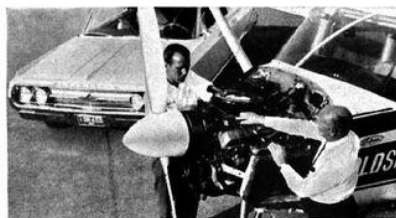
Test pilot Dick Marsh (right) and "Oz" Nelson, chief mechanic, check Jetfire Rocket V-8 Engine installation before historic flight.
